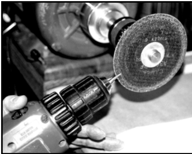
Grinding the shank down to approximately .075"
