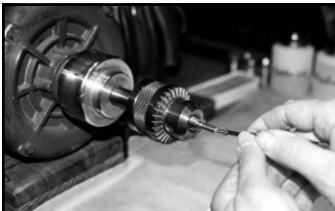
Center Punching the end of the brass stock.
