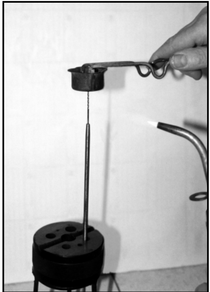
Heating the piece up to brazing temperature, while holding bit in place.
