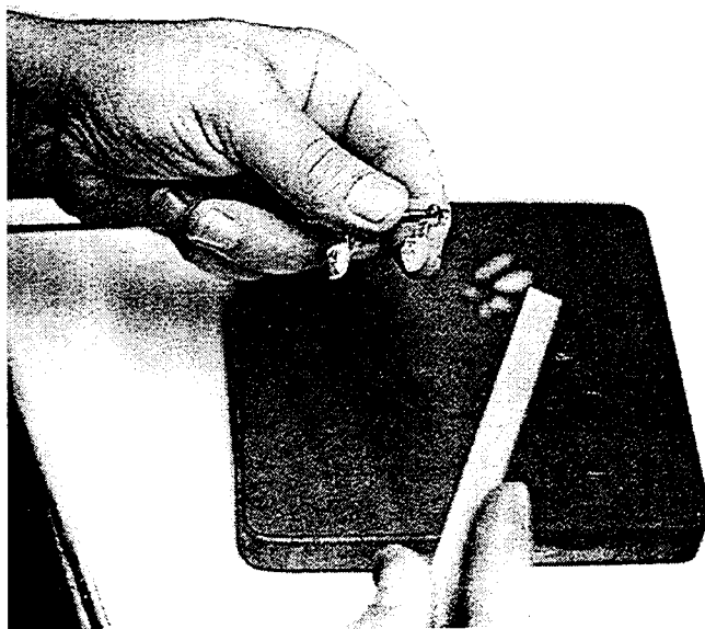
Final sanding and shaping the cork with a sanding stick
