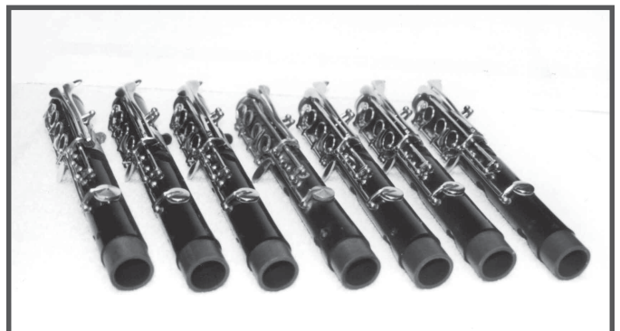
The finished tenon; prior to drilling-out the low F tone hole and cutting the cork slot.
