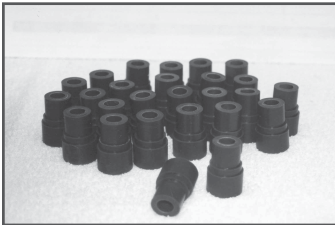
The clarinet bell tenon blank after being bored to .540"
