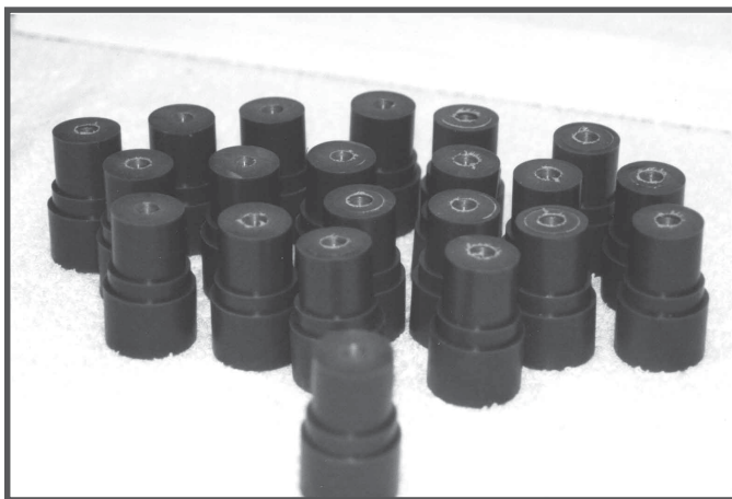
Center bore the small end of each blank
